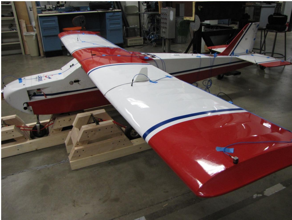
Figure 8. The Super Hauler in the test rig while instrumented with accelerometers.
