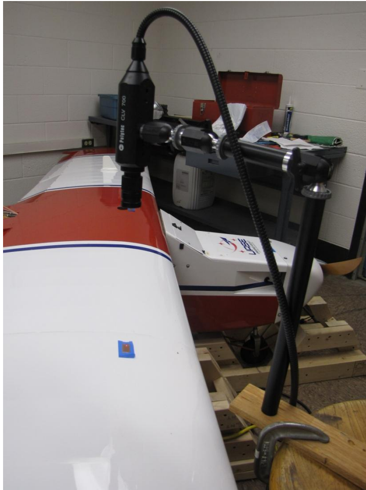
Figure 93. Laser vibrometer testing setup.
